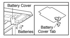
ment, with the negative (–) ends of the batteries touching the springs. Close the battery cover, push up on the tab, and then push the tab forward as shown in the inset drawing. Be sure that the tab locks into place.
